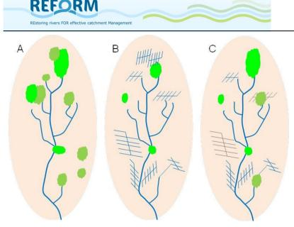
Figure: Hydrological restoration of combined ground water and surface water flows by restoring infiltration capacity and recreating water storage areas. (A: Natural catchment, B: Present situation with a high drainage intensity, C: Restored catchment with water infiltration, reduced drianage intensity, water storage areas (green) and water flow retarding by remeandering).
