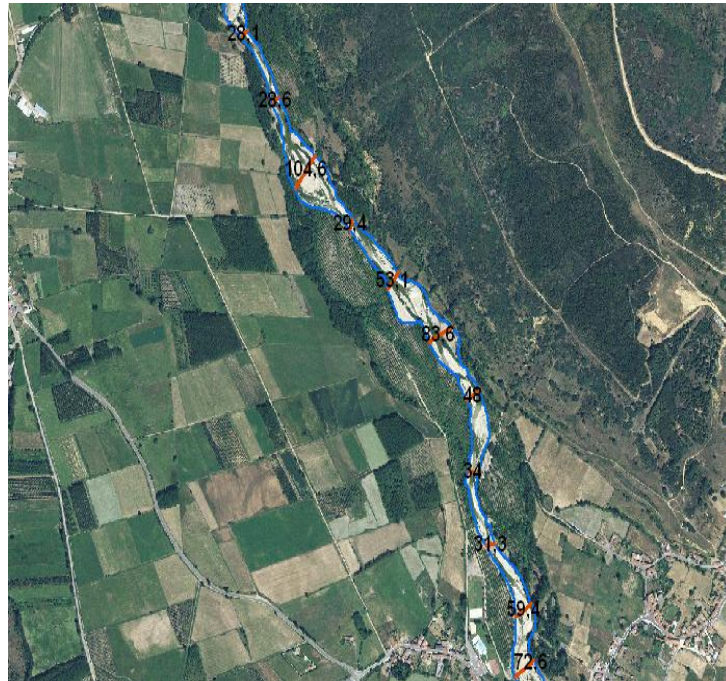
Figure A.5 Active channel width measurements.
