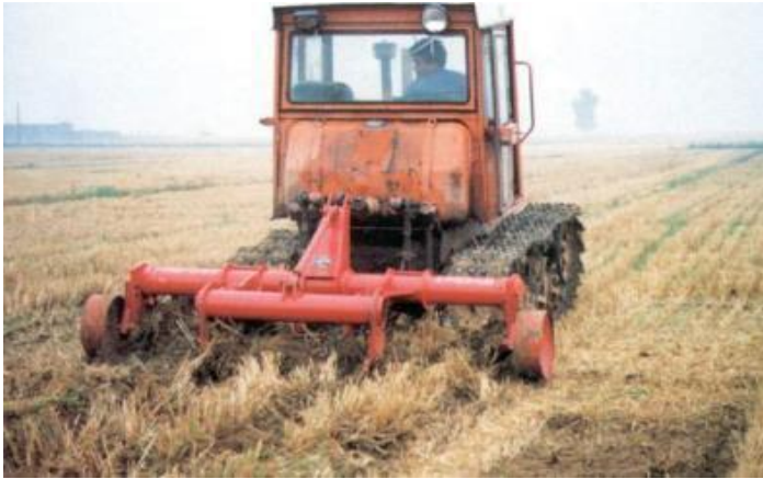
Straw mulching and sub-soiling (Source: Bai, 2014)
